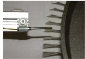
Fiber-based profilometers with miniature probes 3 millimeters in diameter are used to inspect "blisks," bladed disks used in aeronautics.
