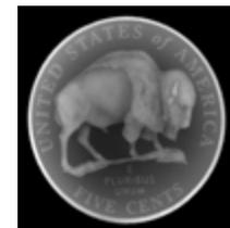
A low coherence profilometer can characterize an object's surface as well as scan the thickness of objects from 10 microns to several millimeters thick with a precision better than 1 micron. *Source: Novacam*
