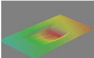
Data is acquired from the worn region of the sample and from the intact region around it, as seen in this 3-D rendering of the scanned surface of a sample (25 by 50 millimeters) after abrasion.
