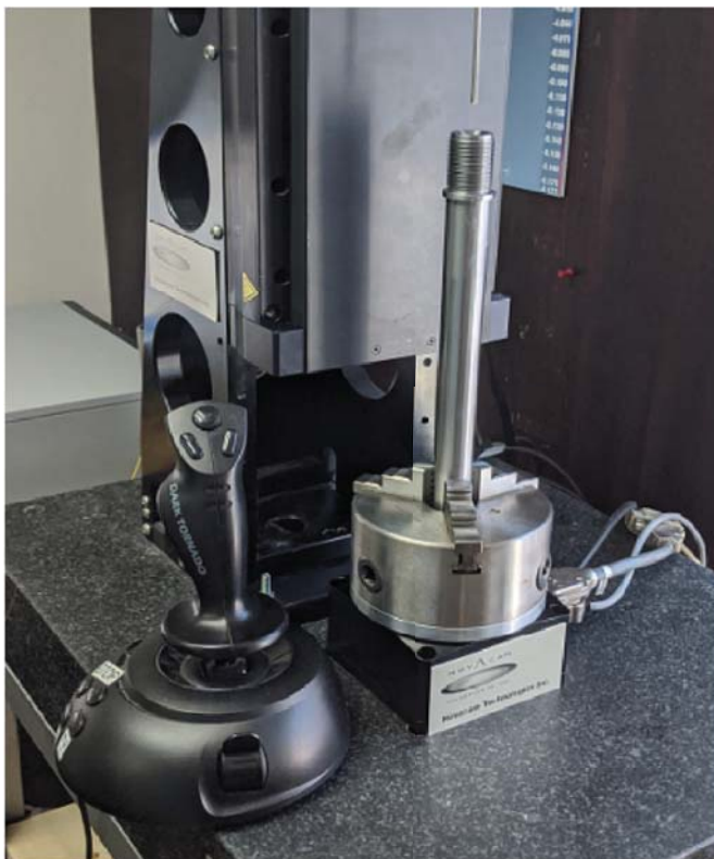
Fig. 1. Novacam measurement apparatus with barrel clamped vertically to eliminate gravity effects.
