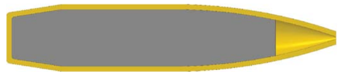
Fig. 4. Sierra MatchKing 140 grain projectile used in modeling and validation efforts.
