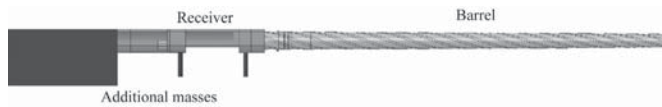
Fig. 5. Full model geometry used in this investigation. Receiver, barrel, and additional masses are shown.
