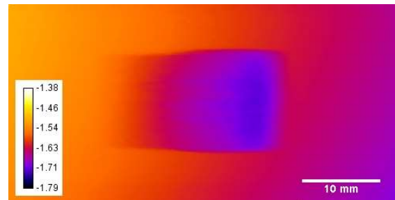
Figure 2: Height image of the surface of the same sample as Figure 1 (color represents depth)
