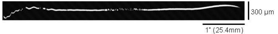
Figure 5: Profile of 6" diameter wafer with unevenly applied thick film of photoresist coating (~250 µm thick, equivalent to approx. 400 µm optical thickness). The X:Y aspect ratio is 10:1.
