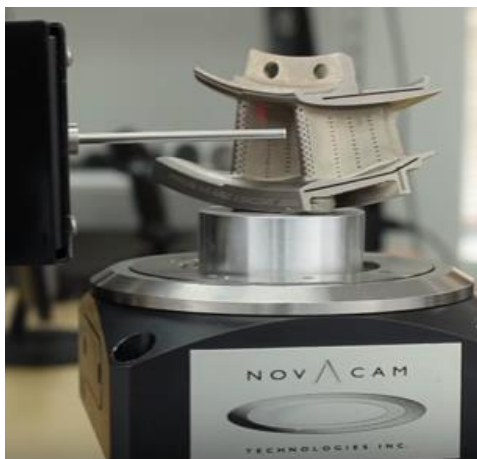
Figure 8: A rotational scanner probe inspects cooling holes on the inner surface of a stator blade.
