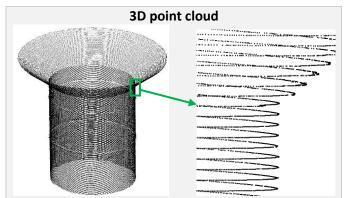
This high-density 3D point cloud comprises over **947,000 3D measurement points**. With the system scan rate of 100,000 Hz, probe rotation speed set to 20/sec, and a spiral pitch of 50  $\mu$ m (~2,000  $\mu$ in.), measurements were 4  $\mu$ m (~157  $\mu$ in.) apart, giving 4,987 3D measurements per rotation. Scan time was 9.5 seconds.
