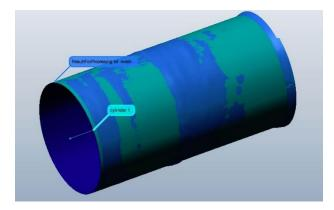
Colour-coded image of dimensional difference between the rivet-hole specification (green) and the measured rivet hole (blue)
