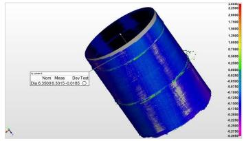
Rivet hole shown as 3D deviation map from cylinder. Users can zoom or pan around the point cloud image, as well as query measurements of features or individual points.
