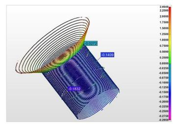
Rivet hole and countersink shown as 3D deviation map from a cylinder.
