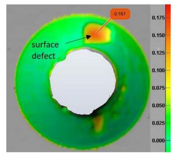
Countersink with a dent (STL view, scale in mm)
