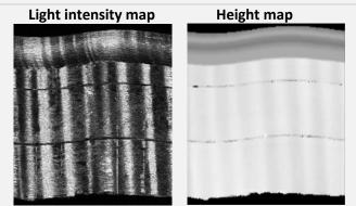
These data sets are generated at the same time as the 3D point cloud file. They represent an unwrapped view of the rivet hole ID and may reveal evidence of defects such as chatter (seen as vertical stripes) and inter-laminar defects. The 3D point cloud is useful for both interactive and automated 3D analysis of the measured surface and for calculating 3D GD&T parameters.
