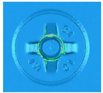
Installed rivet head measured with the SURFACEINSPECT system and viewed as an STL file in InnovMetric PolyWorks Inspector.
