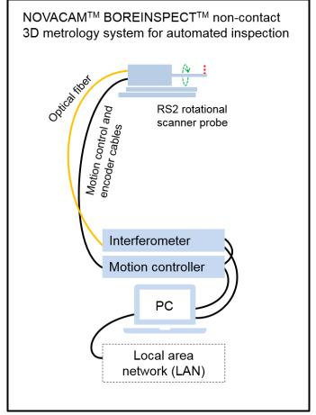
Simplified diagram of the BOREINSPECT system, where the RS is set up as robot end-effector (not to scale)
