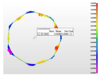
Drill bit chatter on a circular profile of the rivet hole
