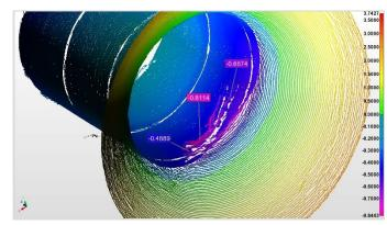
Rivet hole and countersink shown as 3D deviation map from cylinder. A burr defect (pink) is evident on the rivet hole ID.
