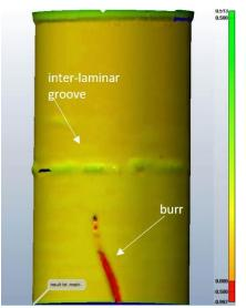
Rivet hole ID with an inter-laminar groove and a burr (STL view)
