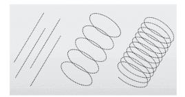
With the SURFACEINSPECT system, the light beam traverses the lens field of view (FOV) rapidly and following a raster pattern.
