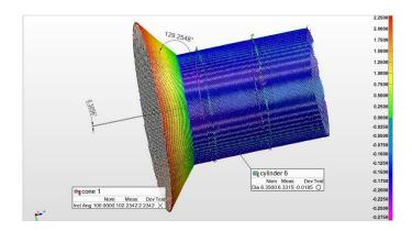
Rivet hole and countersink angle measurements
