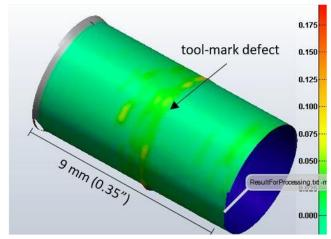
Tool-mark defects at the interface of material layers (STL view)
