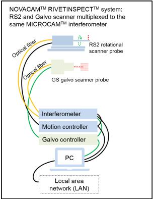
Simplified diagram of the RIVETINSPECT system where both the RS and GS are set up as robot end-effectors (not to scale)
