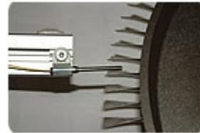
On the other hand, blisks are more expensive to repair. If a blade is damaged, the entire part must be replaced. As a result, blisks get an erosion-resistant coating so the blades last as long as possible. Though measured in microns, the thickness of this coating is critical to its effectiveness.
