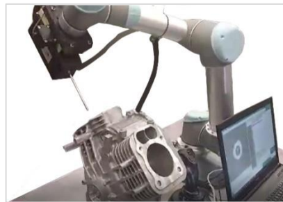
The rotational scanner (RS) is mountable on a variety of precision stages, gantries, and robot arms
