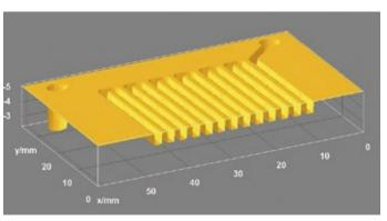
Fig. 1: 3D rendering of a fuel cell bipolar plate, an example of high-aspect ratio imaging
