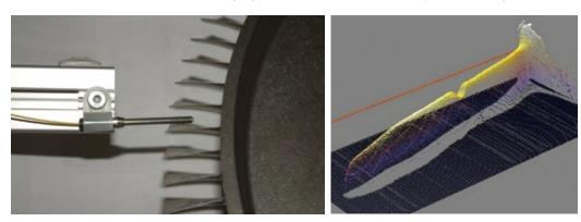
Fig. 3: A fiber-based probe mounted on a scanning mechanism inspects the surface of blisks (bladed disks used in aeronautics). A leading edge of a turbine blade can be accessed and inspected.
