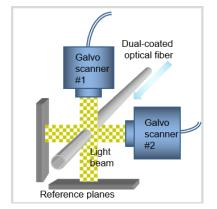
**Figure 3:** Dual probe setup for long profile scanning of optical fiber. With continuous scanning, the entire fiber cross-section is acquired in real time.
